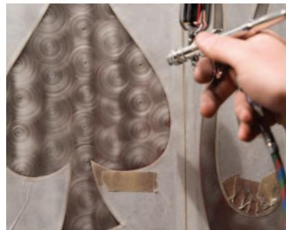
cure overnight, and then Scotchbrite® and add as many wet coats as you wish. Using this method, a protective barrier is established between the wet clear and your shiny aluminum. We experienced great results with House of Kolor's UC-35 fast-drying clearcoat. I also prefer to perform this effect on either small panels or integrated into graphics. Trying to chrome an entire car or a hood is not only a little overkill, but it tends to look streaky and blotchy.
