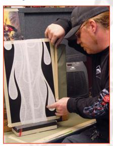
STEP 2. I masked off a few flames on the black panel so you can see how the stencils are used for excellent background filler and graphic effect.
