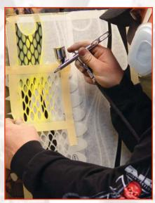
STEP 3: Using one of the inner repeating patterns, I airbrushed lemon yellow in one of the flames. While all of my stencils are hand-drawn, we did use a computer on the inner pattern of this stencil, just like the diamond plate, so that you can easily overlap and layer the stencil to fill any design size.
