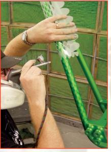
STEP II: As a cool closer, I wanted to show you how easily the stencil wraps around things. For the smaller scales, I used the other two edges of the stencil. All you have to do is slide the curved stencil down the tubes of the frame to give a killer all-over scale effect that would otherwise take forever to mask, and would look terrible if freehanded.
