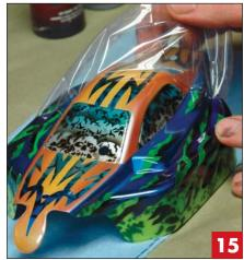
**15.** One of the most rewarding aspects of this process is removing the protective coating from the body, after which the design literally comes to life and looks terrific. Of course, don't be like me and forget to remove the coating, as I did the first time I painted a Lexan™ body. Sadly, I had to remove all the logos and pinstripes I had painted and start over!
