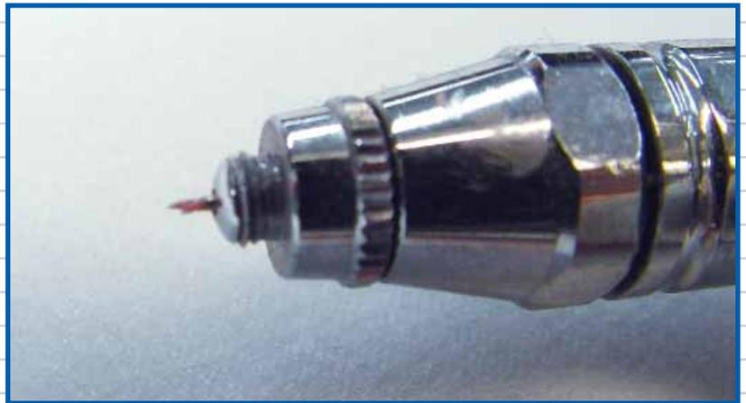
**Fig 4:** An example of a properly cleaned needle. Note that the nozzle, or needle cap, has been removed for cleaning. Gently unscrew the nozzle and treat these small parts, particularly the needle, carefully. Even slight damage can make your paint go haywire. A soft cloth or tissue wetted with cleaning solution, or very gentle scraping with a fingernail, can remove dry paint from the needle tip. But again, go slowly and exercise care.
