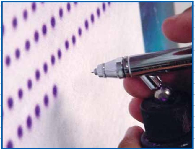
**Fig 6:** Position the airbrush nozzle between one-half and one inch from the surface and begin painting. Keep the airflow constant. Roll the trigger on and off to make a dot. Nail it in one shot. In this sequence, I've kept my nozzle cap off the airbrush to facilitate cleaning of dried paint from the needle tip.
