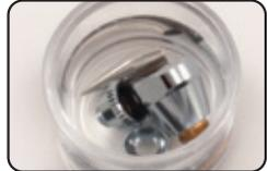
**4c.** Using an extra small cleaning brush dipped in Medea Airbrush Cleaner, scrub your nozzle, nozzle head cap, needle cap and nozzle cap.
