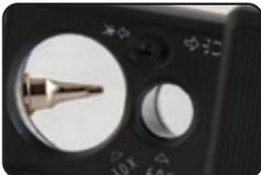
1. Look at your nozzle for cracks or dents or to check for distortion.
