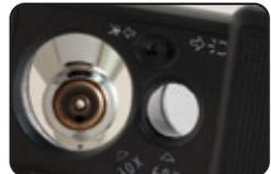
3. Check for paint debris inside airbrush paint passages.
