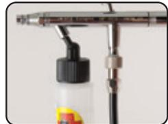
**1c.** Spray the cleaner or water through the airbrush until it sprays clear. Spray into an overspray pot or paper towel.
