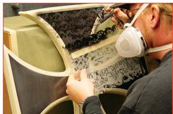
Step 2: Using the skull lineup on the top of the *Multiple II* stencil, begin layering skulls, staggering them along the cross. BC-25 House of Kolor black basecoat contrasts nicely with the reflective ghost chrome. The strip of masking tape keeps the overspray from getting into the other stencil areas.
