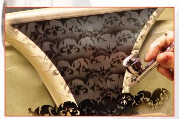
Step 3: Being careful to not kill the aluminum effect, hit the stencil lightly with the black. The nice thing about stencils: If you don't apply enough paint, you can always line it back up and shoot the sucker again.
