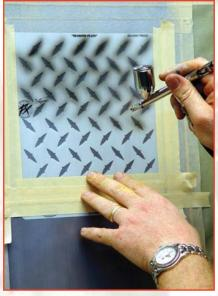
STEP 5. Loading the airbrush with House of Kolor BC-25 basecoat black, I lightly dust the individual diamond shapes with an Eclipse HP-CS. Don't apply too much paint at once or the stencil will get too wet, unusable, and may cause the paint to creep underneath.
