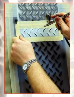
STEP 10. With the black finished, I then use HoK BC-26 basecoat white. The bottom half of the Diamond Plate has some half stencils that are used for the highlights. Lining up one row of diamonds at a time, I spray in the top highlight of each.
