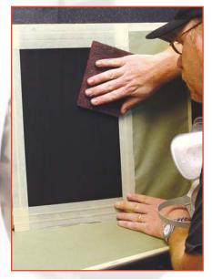
STEP 1. After masking off the powder-coated panel, I scuff the heck out of the surface. Normally, I would just scuff it enough to get the paint to stick, but in this case I'm going to use some of ALSA's Ghost Chrome for a brushed-aluminum effect. The extra scratches I give the panel make the effect even more realistic.
