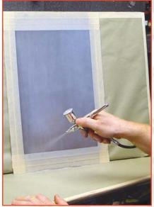
STEP 2. Using the new Iwata trigger airbrush, I spray on a few layers of Ghost Chrome. This new trigger side-feed model sprays the Ghost Chrome pretty killer without layering it too heavy. This airbrush is also beneficial to painters who are used to using sprayguns. With the Ghost Chrome layered evenly, the panel now looks just like a brushed sheet of aluminum.
