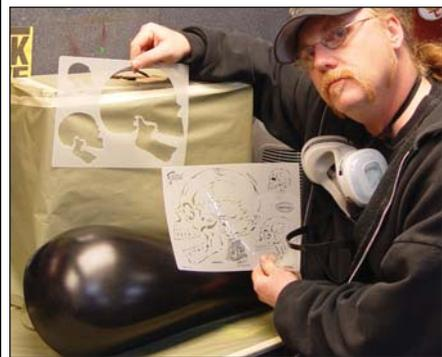
**STEP 1.** Coast's tank blanks come gel-coated. To prep the surface, I sanded the gelcoat with 220-grit sandpaper, then applied primer, based in black, and cleared it with House of Kolor UC-35 clear. Artwork always comes out nicer when it's applied over sanded clear. Notice the negative and positive stencils for the profile skull.
