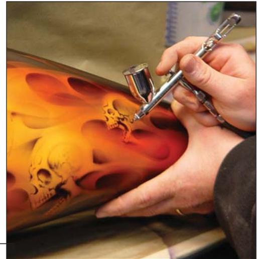
**STEP 9.** Using the same violet/tangerine kandy mix, I rendered the details of the skull with the new Eclipse CS Kustom airbrush. You must connect all the stencil lines and soften them enough so the final image doesn't look like a stencil was used. With proper stencil application, the final result should look freehanded.
