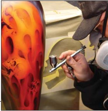
**STEP 10.** I switched back to kandy apple red and blended more color into the flames. This also softens the tight details and eliminates any leftover violet that may have been showing through. Even when working on small projects, you should always wear, at the very least, a dual-cartridge active charcoal respirator.
