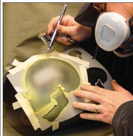
**STEP 2.** Using a few pieces of tape to hold down the stencil and to prevent overspray, I lightly sprayed SG-101 lemon yellow for my base color. I mainly emphasized the outside edge and details of the stencil, leaving the center alone for later.
