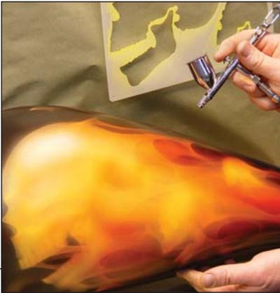
**STEP 7.** With the yellow sketching completed, I switched gears and separately mixed a batch of KK-08 Tangerine and KK-11 Kandy Apple red—be sure to mix them only 20% by volume to the SG-100 intercoat clear before reducing. I then layered the kandy basecoats over the yellow for added color and killer depth to my fire.
