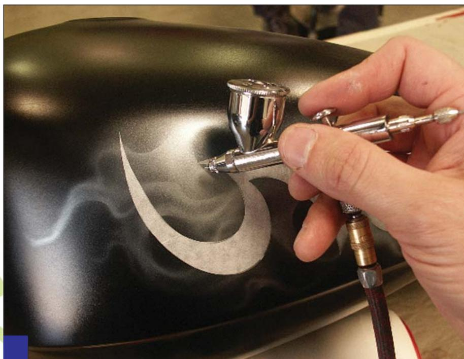
**STEP** I then used House of Kolor BC-26 white to freehand airbrush realistic fire and smoke as a good backdrop for the tribals. Be sure to render the fire all over the masked tribal. Any area left unsprayed around the cut edge will look unresolved when unmasked. The more paint, the more contrast.
