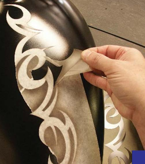
**STEP** With all the tribals airbrushed, I followed the stenciled spray pattern with a sharp X-Acto knife, and removed the surrounding negative space of the design, leaving the positive portion masked (you can just as easily remove the positive section and spray the actual tribal, but that's another article) Be careful not to cut too deep or you'll gouge or score the tank's surface.
