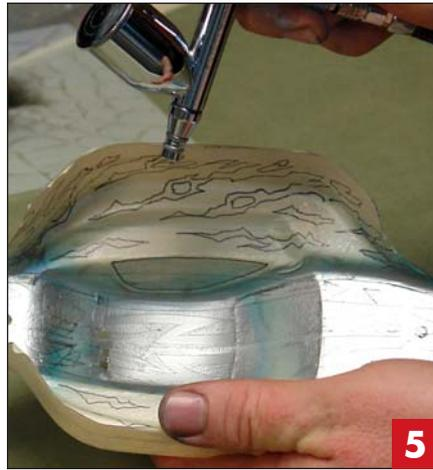
**5.** After the kandy dried, I layered in a few light coats of House of Kolor's new Kosmic Krome Aluminum effect to give the tribal graphic a killer aluminum look. Remember, when spraying these graphics on Lexan™, you have to work in reverse order of how you would normally paint a metal surface. Therefore, the aluminum application on lexan is the backing color; the last color sprayed instead of being the first.
