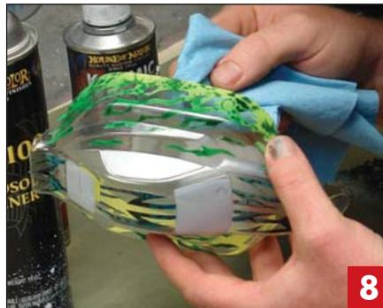
**8.** After unmasking the remaining areas of the car, I wiped down all the overspray with House of Kolor's KCA-100 pre-cleaner. This stuff is killer and comes in an aerosol can. I spray KCA-100 into a rag first and then wipe out any bleeds or defects in the paint job. It's also great for removing any residual tape adhesive.
