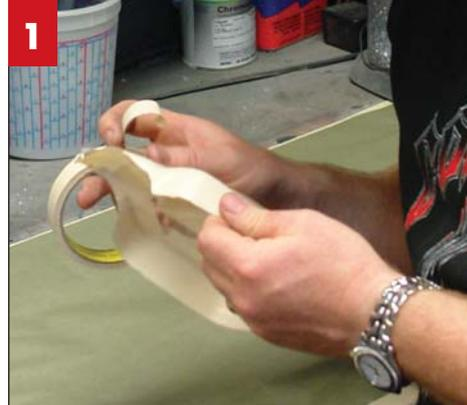
**1.** No matter what scale or brand, the first step is to use an X-Acto blade to clean the edges of the RC body, cut out any necessary holes, and you're ready to paint. Before spraying, I like to apply a layer of 3M automotive-grade masking tape. Keep overlaps to a minimum, and this will give you a great masking surface.
