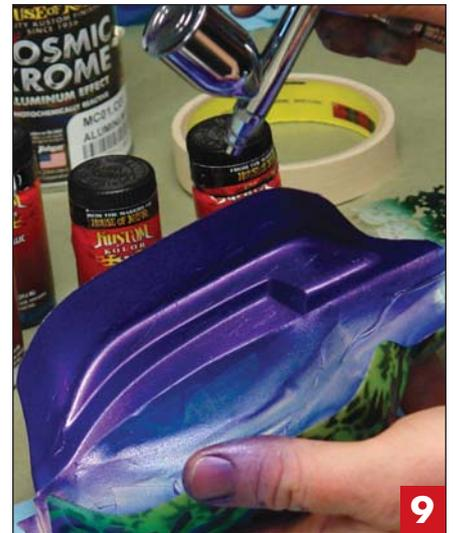
**9.** After masking off an underlying two-tone with 1/2-inch masking tape, I rendered a cool fade using Kustom Kolor's Metallic Blue and Pavo Purple. Backing up a step, while you can't see the drop shadow, I did airbrush one in before any color was applied to this two-tone. Remember, everything is backwards.
