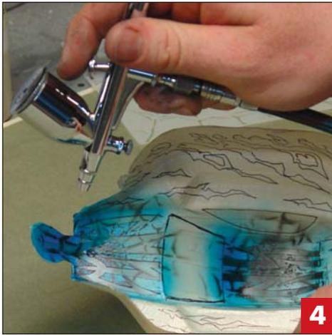
**4.** With the *Spider Web* design airbrushed, I added a blue fade using SG-100 and KK-04 intercoat clear. Because I used standard House of Kolor basecoats for this step, it was necessary to airbrush a light coat of AP-01 adhesion promoter ahead of time.
