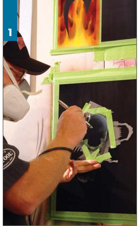
**1.** Starting with House of Kolor BC-26 basecoat white, I airbrush the basic shape of the skull with the original *Skullmaster Frontal* stencil. Masking off the areas around the skull itself not only helps reduce overspray, but also helps the stencil to adhere better to the surface.
