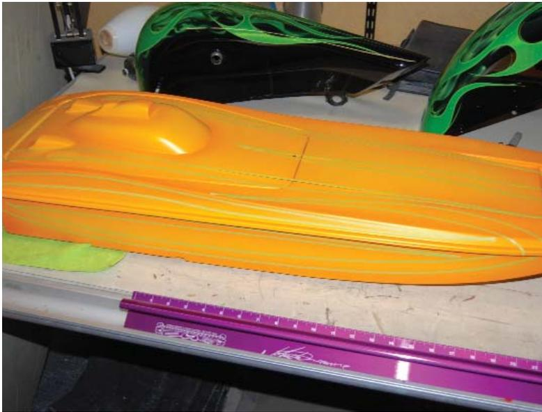
Notice that I followed the contours of the boat with 3M 1/8-inch green fine-line masking tape. This should serve to add a sense of speed and movement to enhance the already fast look of the boat.
