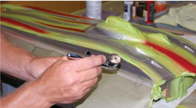
Before spraying Auto-Air's Fine Aluminum (#4101), I covered all the red areas to avoid contamination. Then, I airbrushed Semi Opaque Black (#4220), thinned 50-percent, to achieve a very light fade around the edges of the Aluminum. I'm just off the tape's edge, allowing the overspray to do the fade. This adds more dimension to the job.
