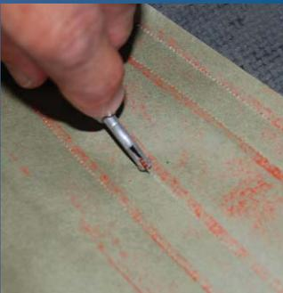
8. I removed the paper, placed it on a semi soft surface, and produced holes on the inside track of the tape with a fine pounce wheel.
