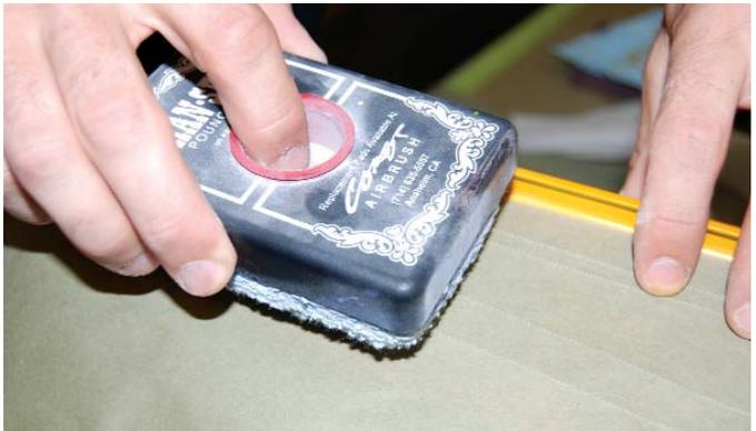
I flipped the paper over, lined up the design to the other side, and used a pounce pad filled with blue chalk to pat over the holes created by the pounce wheel. I removed the paper and followed the blue chalk dots with 1/8-inch fine-line tape.
