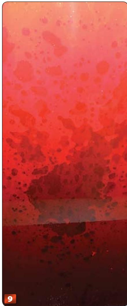
I cut several pieces of aluminum blanks—commonly used in the sign industry—8-inches by 24-inches, scuffed them with a red Scotch-Brite pad to establish a tooth to the surface, and applied a black automotive base coat with a spray gun.
