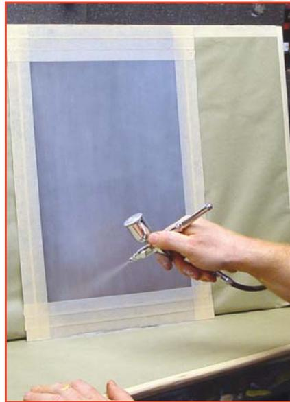
**STEP 2.** Using the new Iwata trigger airbrush, I spray on a few layers of Ghost Chrome. This new trigger side-feed model sprays the Ghost Chrome pretty killer without layering it too heavy. This airbrush is also beneficial to painters who are used to using sprayguns. With the Ghost Chrome layered evenly, the panel now looks just like a brushed sheet of aluminum.
