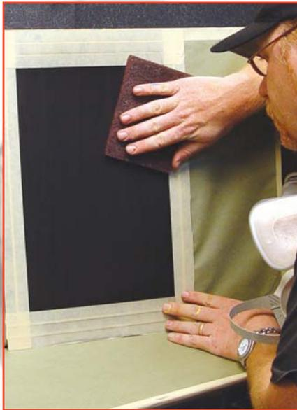
**STEP 1.** After masking off the powder-coated panel, I scuff the heck out of the surface. Normally, I would just scuff it enough to get the paint to stick, but in this case I'm going to use some of ALSA's Ghost Chrome for a brushed-aluminum effect. The extra scratches I give the panel make the effect even more realistic.
