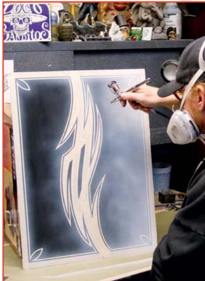
**STEP 2.** With the graphic masked off, I airbrushed a layer of House of Kolor's HoK BC-26 white with an Iwata TR-1 trigger gun, applied in a graduated pattern to create a slight smoke effect throughout. This provides a good background. Light on the right, and darker on the left to do the stenciling over.
