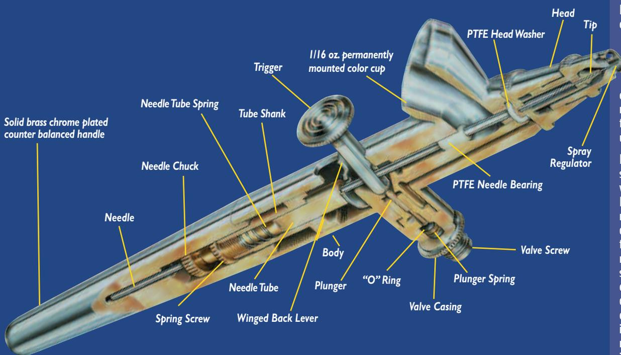
Before choosing an airbrush, consider the factors unique to your particular situation. What type of work will the airbrush be used for? What type of materials will be sprayed through the airbrush? What is your level of experience? etc? The list of terms, the cut-away airbrush diagram, and the reference chart will help you select the best airbrush for your intended application. But if you have questions, you can always call us at 1 (800) AIR-BRUSH.
