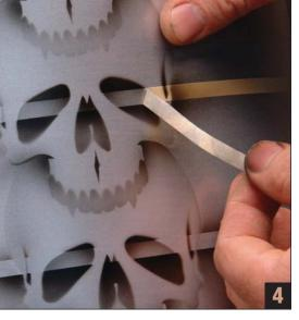
**4.** The 3-D effect was accomplished by combining a little tape work with the stencils. The key to using a stencil successfully is to make sure that it's clean, does not look like a stenciled effect, and that it saves you more time than not using one. So far, so good.
