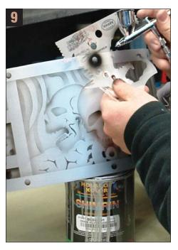
**9.** Instead of digging up a circle template, I used *Screaming's* skull stencil. There are a number of different-sized circles in this stencil, and they work great for rendering rivets and screws. When spraying these rivets, I hit the bottom of the circles more to give the illusion of shadow.
