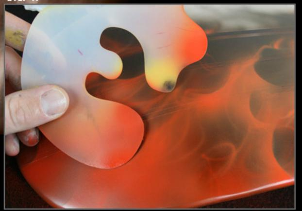
The AIRSICK "ARSON SET" contains an assortment of various sized French curves. By matching up the right sized curve to our fire, we can begin to make the edges harder and add more definition to the flames.
