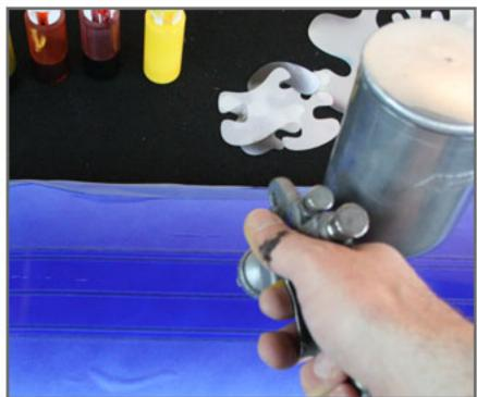
Build up your color with a multiple light passes. You do not want the paint to build up to quickly. This could lead to issues when the masking is pulled away from the skate deck.
