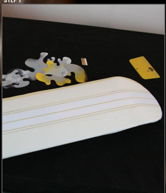
Before starting with the design, the skate deck has been properly sanded, primed and base coated with House of Kolor Base White (BC26). Proper prep will ensure that there are no issues with peeling paint after masking. With the board properly measured out, we proceed to tape off a simple racing stripe design (STEPS 1 & 2).
