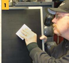
1. After scuffing the powdercoated black metal blank with a red Scotchbrite pad, I back-masked the panel with Ultramask, a new masking product from Artool. Unlike AutoMask, Ultramask has the advantage of being transparent. It also comes with a backing paper for use in cutting your own stencils on a plotter. And unlike frisket, Ultramask is solvent-proof and will stick to basecoated and clearcoated surfaces.
