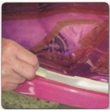
**STEP6**After the fades dried (I also applied two coats of intercoat clear over the fade) I unmasked the inner border that will have a candy yellow-to-orange fade.
