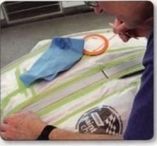
**STEP 8**Here you can see the magenta and purple fades. The side panel has the additional taping finished and the top is getting an inner 1/8-inch tape line.
