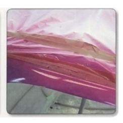
**STEP 4**Starting with magenta candy concentrate mixed with intercoat clear, I carefully faded the magenta, front to rear, using a SATA Mini-jet gun. At the rear I mixed purple candy concentrate and started building color
