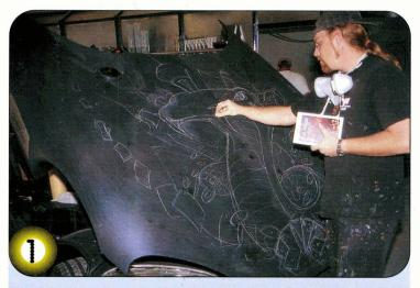
**STEP 1** After the clearcoated midnight blue pearl (applied by Dion over the original red) is sanded down, the Viper has more of a flat black look. For the initial design sketches, I use a piece of white construction chalk to "rough in" the snake and the surrounding Vegas strip.
