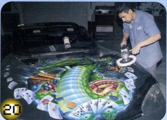
**STEP 19** After giving the last clearcoat 24 hours to cure, Dion prefers to do the fun part on his own. Color sanding with 1500 grit wet/dry sandpaper, the surface shine is knocked down in preparation for the final buffing, polishing, and waxing.
